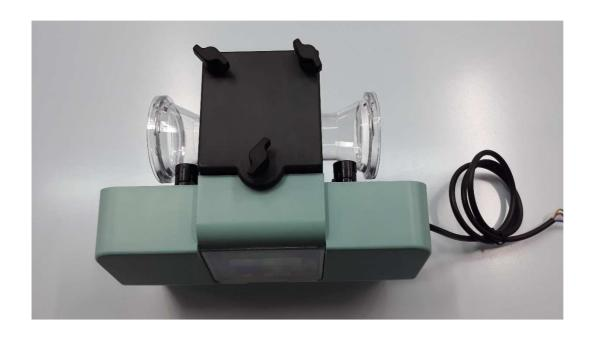
**Step 2.** Remove the 3 plastic nuts and the black upper cover. Disconnect the connector cables from the cell one by one (2 blacks, 1 white).
