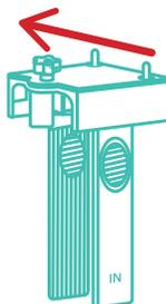
**Note:** The arrow in the picture above indicates the correct direction of the water flow.
