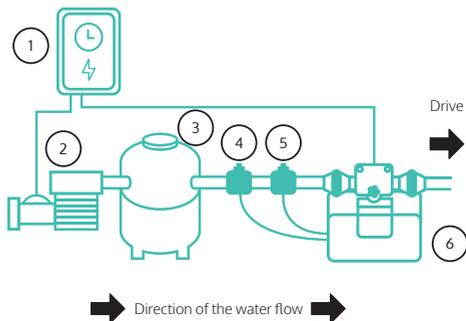
**Attention:** Make sure you have a long enough length of pipe to install the electrolysis cell and flow sensor.
