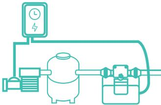
The electrical connection must be made in such a way that the QUICKSALT chlorinator is started only when the filtration pump is in operation. Therefore, be sure to carefully choose the right contactor output.
