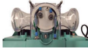
**Attention:** Please, ensure that the connection cables between the cell and the control unit, are placed over the green mark.
