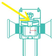
**2)** On the inside of the housing, you will notice that there are two baffles marked IN and OUT. These deflectors can be interchanged with each other.
